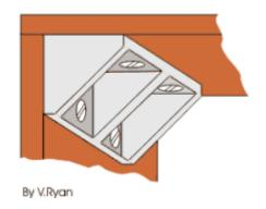
**RIGID JOINT**: These are normally moulded in plastic which makes them strong. Screws pass through the four holes which hold the sides at each corner firmly together
