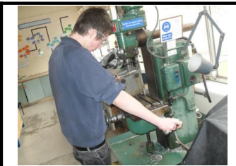
Explanation: This is a picture of me milling me aluminium cast docking part
